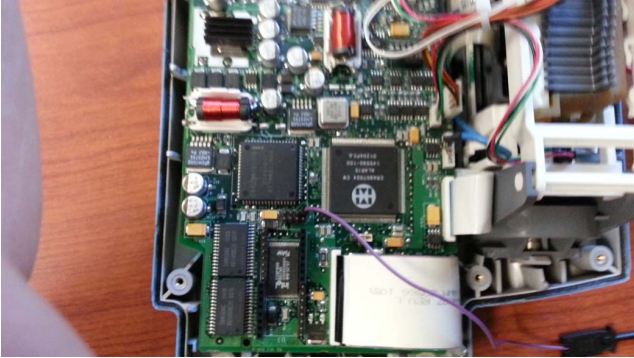
Fig. 3. Board Layout of the Alaris SE 7132. Redundant SRAM chips on left, CPU top-middle, flash between header pins, ASIC top-right.
